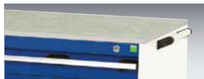
Lino 20mm thick with lino worksurface bonded to particle board core. Trolley height 890 / 990mm.
