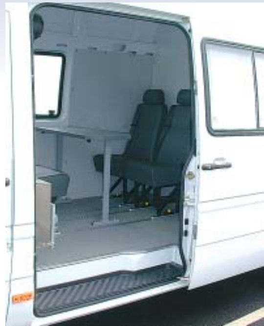
Crew cab facilities with fold down table and heated hand wash.
